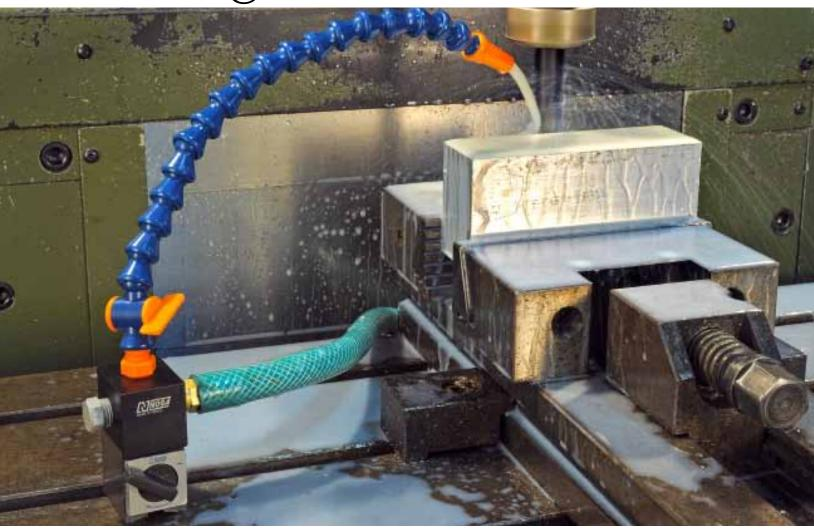
**NOGACOOL** consists of a manifold & Loc-Line® flexible hose with a nozzle on top and a valve at the bottom, assembled on the powerful on/off Popeye magnet.
