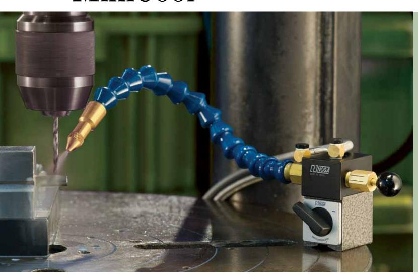
**NOGA MINICOOL** uses the VENTURI principle to spray an air and liquid mixture. It consists of the following basic parts:
